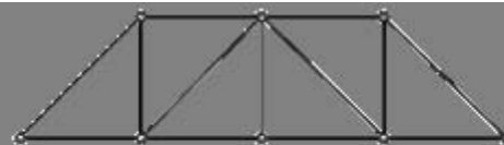
Howe Bridge Truss
