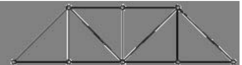
Pratt Bridge Truss
