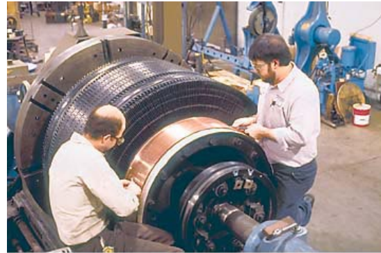
220 KW Exciter Armature for an Electric Utility generator
