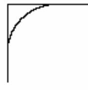
two lines filleted with the No Trim option set
