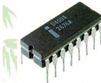
Intel 4004 with 2300 transistors inside
