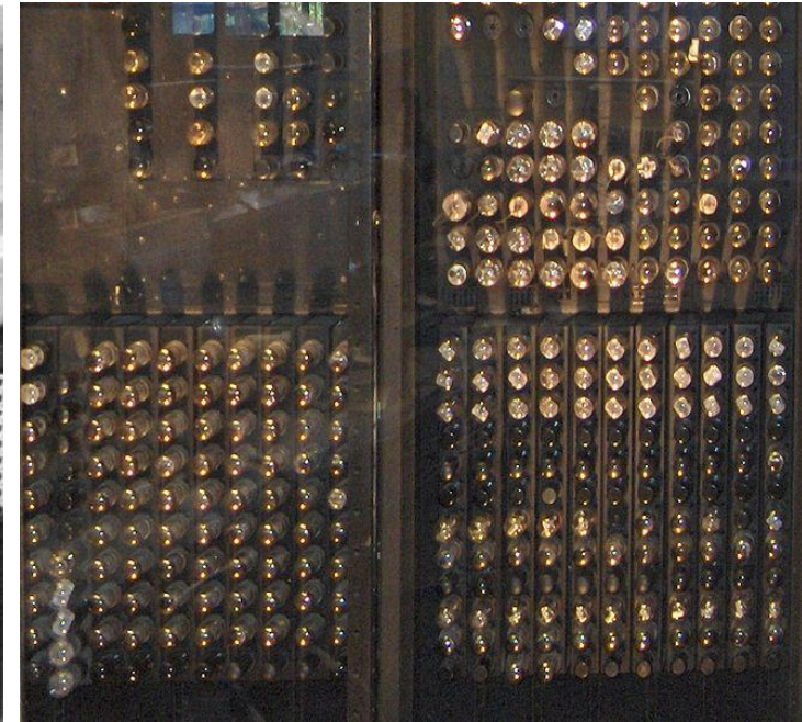
Detail of the back of a panel of ENIAC, showing vacuum tubes
