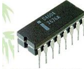
Intel 4004 with 2300 transistors inside
